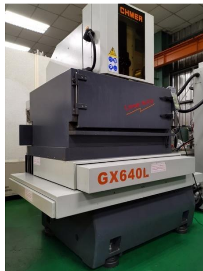
Figure 11 CHMER-GX640L wire electrical discharge machine
